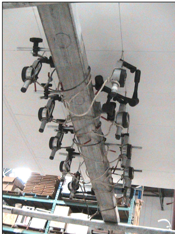
Figure 2. Deflection Measurement Apparatus
